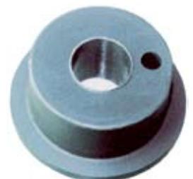
(inset center) Machining G10 fiber-glass spacer.
